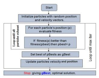
Fig. 2. Particle swarm optimization flow chart1
