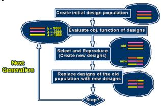
Fig. 1. Genetic algorithm flowchart
