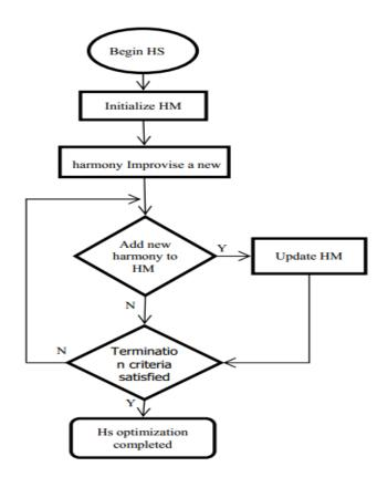
Fig. 3. How the harmony search algorithm works
